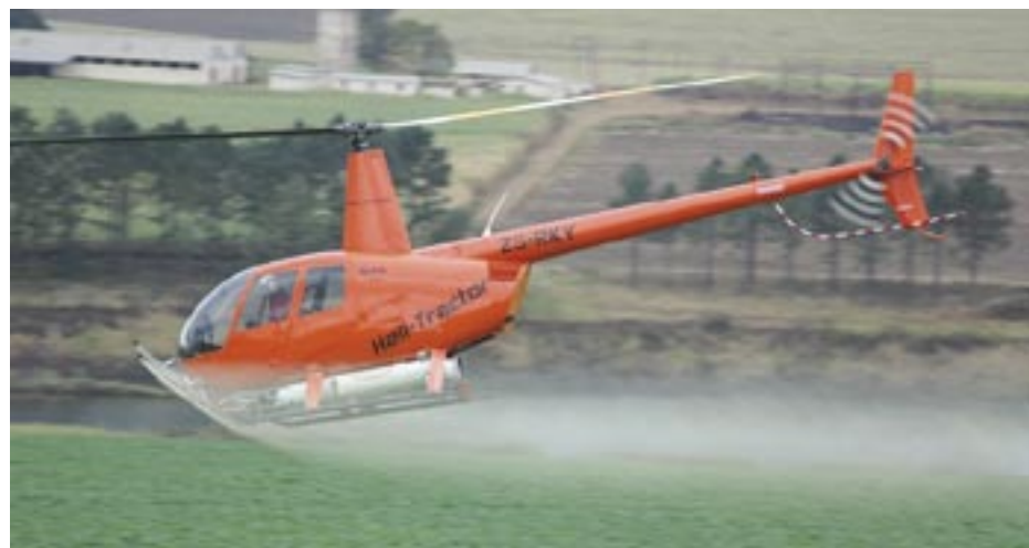
This photo demonstrates that no chemical is being deposited on the tail and rear section of the R44. This helps prevent corrosion, sugarcane in the background.
