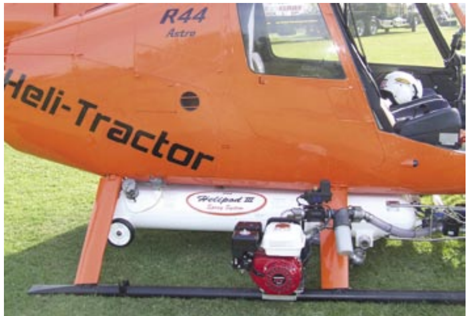
The 5.5 hp Honda/Pacer transfer pump mounting on right side of R44 with the Helipod unit. Note wheels on tank for easy of removal.
