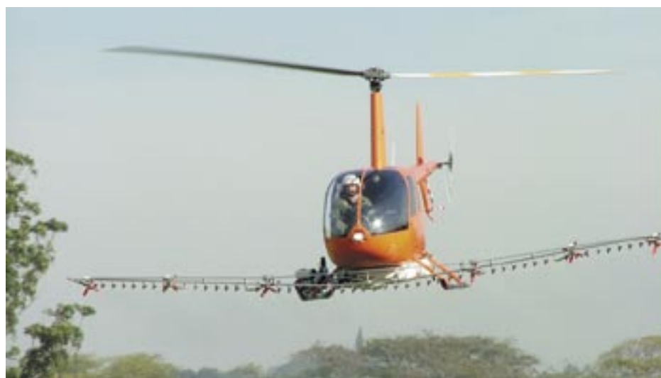
The 80% boom length installed with six Micronairs and TeeJet nozzles. Note the streamline Helipod unit mounted to the belly of the R44.
