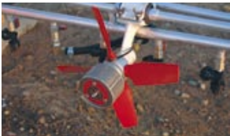
The Micronair rotary atomizers and the TeeJet hydraulic nozzles mounted on the same boom.
