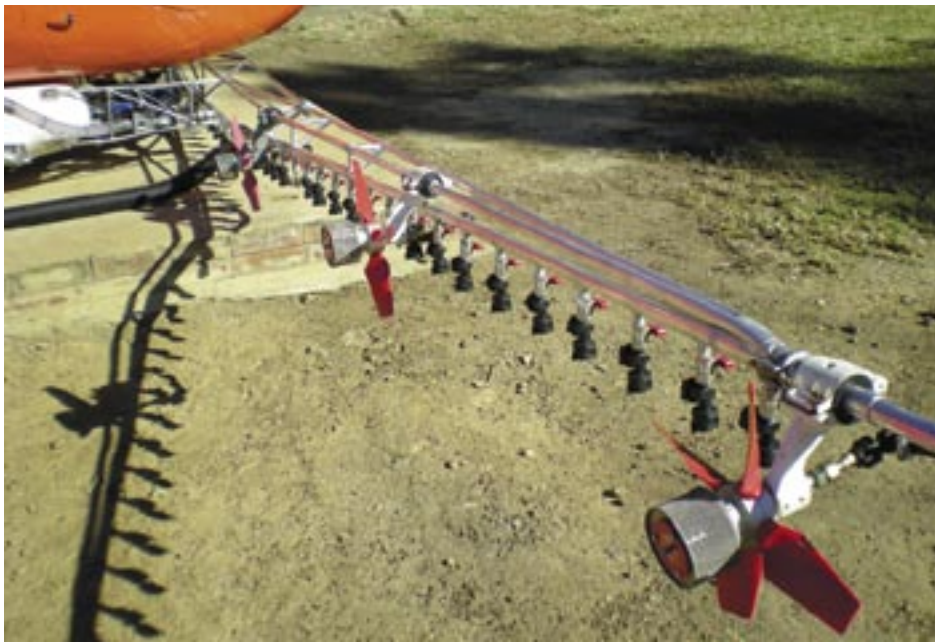
The Micronair rotary atomizers and the TeeJet hydraulic nozzles mounted on the same boom.
